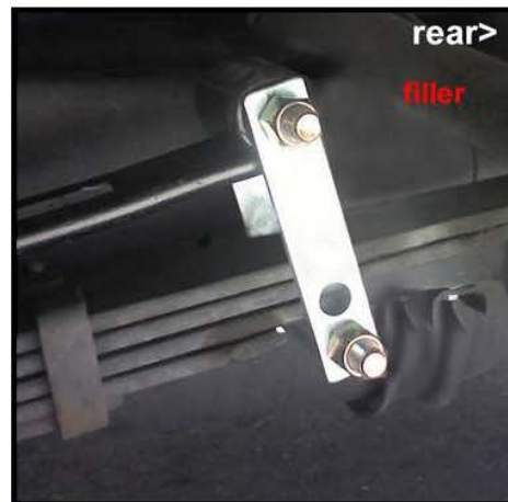
Mount spring eye forward of fuel filler line
