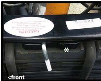
Place PSP-7 on top of spring plate flat side up facing, with groove toward the front
