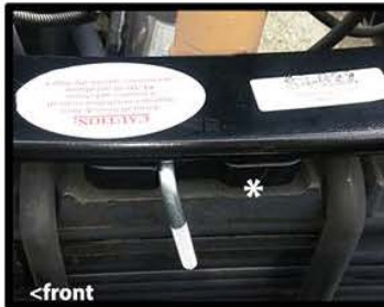
Place PSP11 on top of spring plate flat side up facing, with groove toward the front
