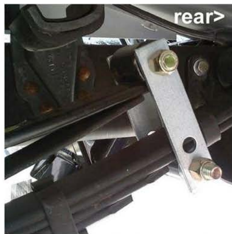
install spring eye bolts threads out
