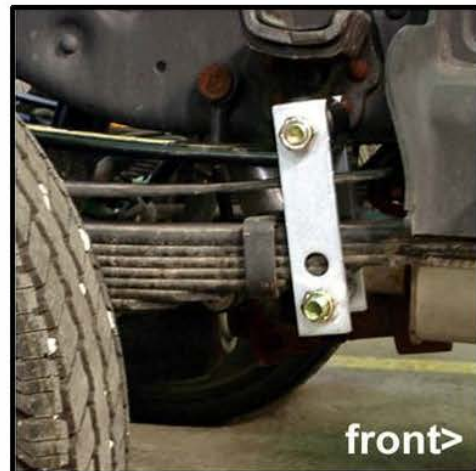
install spring eye bolts threads out
