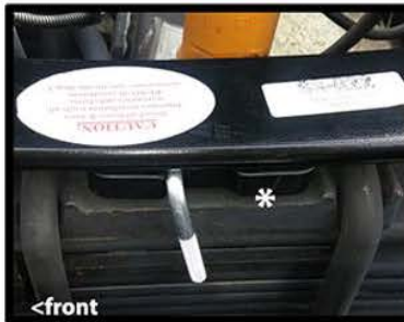
<front Place PSP11 on top of spring plate flat side up facing, with groove toward the front
