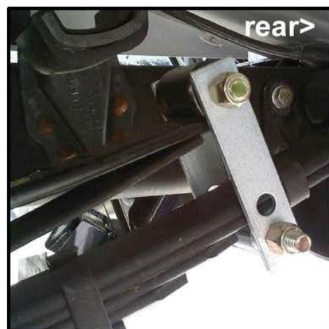
install spring eye bolts threads out
