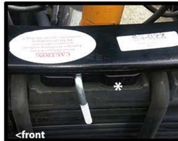
Place PSP 7 on top of the spring plate with small knobs facing down with the hold-down ubolt under the PSP -7 between the center knob and the two knobs oriented toward the front of the truck.
