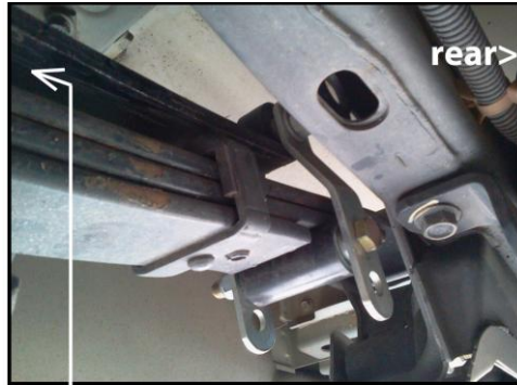
Remove rear rebound clip bolt and roller
