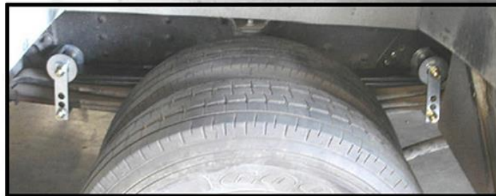
Place PSP11 on top of spring plate flat side up facing, with groove toward the front
