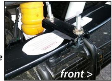
front > "Spring Lock-Down Kit" installed toward the front of the truck between the PSP7 poly pad and the SuperSpring
