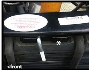
Place PSP-7 on top of spring plate flat side up facing, with groove toward the front
