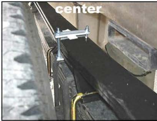
SuperSprings Mounting Kit # MXKT Installed
