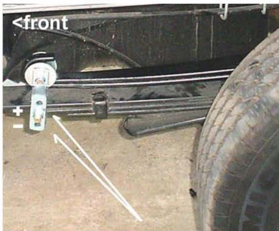
Adjustable pre-load and ride height [fomt rear]
