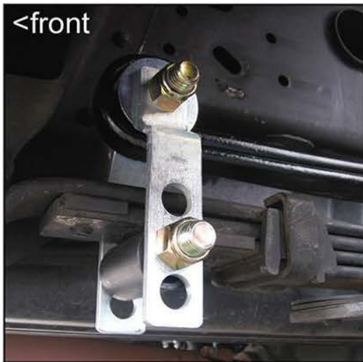
front ~ spring eye bolt threads out
