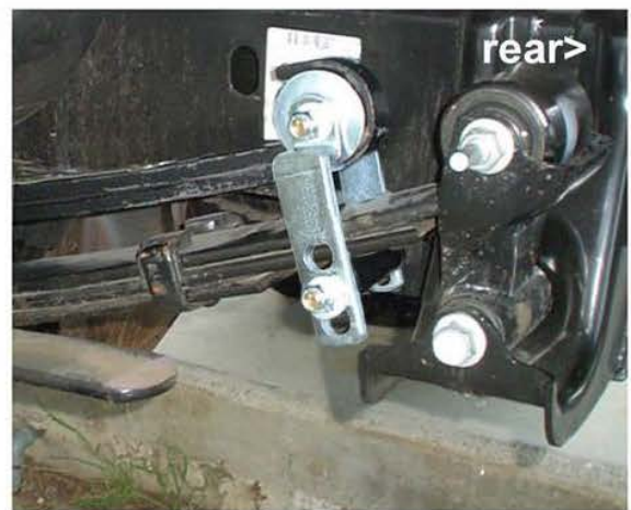
Adjustable pre-load and ride height [fomt rear]
