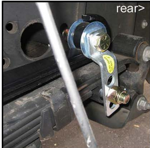
front & rear ~ adjustable preload
