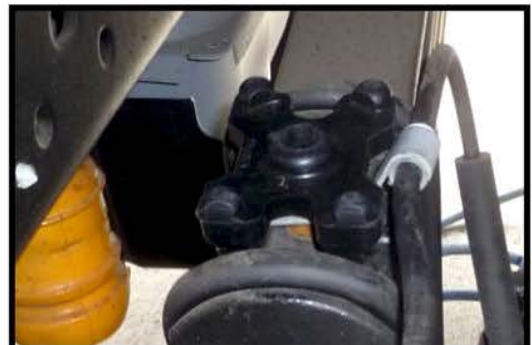
2011~2013 brake cable holder adjusted to allow space for installation
