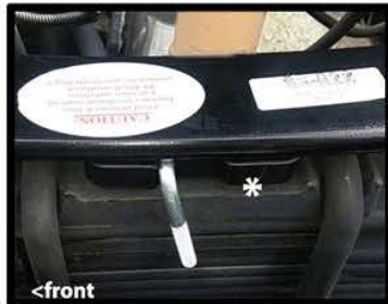
PSP 7 with hold-down clamp assembly
