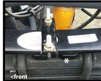
<front Install the SuperSprings as pictured below, then thread the channel crossplate on to the ubolt. Tighten securely.
