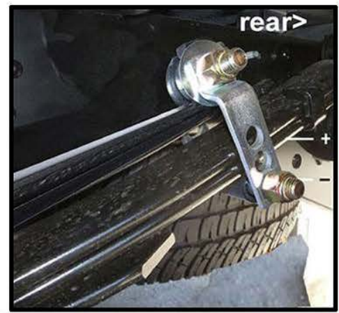
2011~2013 brake cable holder adjusted to allow space for installation
