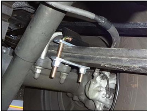
Brake cable routed between OE springs and SuperSprings
