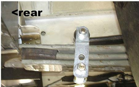
Factory springs are 3 leaf non-parabolic steel springs
