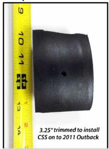
SumoSprings installation possible with or without removal of strut from the vehicle.
