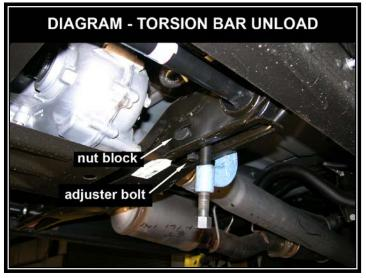
Load the torsion bar then remove the adjusting bolt and nut block. Unload the bar.
