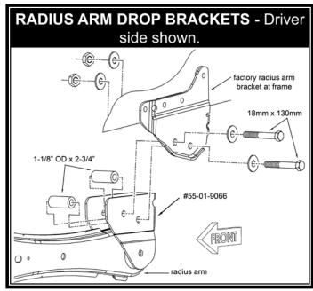
axle. □□ [SEE DIAGRAM] Position the radius arm drop bracket (#55-01-9066) inside the factory mount on the frame, as shown. Align the drop bracket's side and rear mounting holes with the existing holes in the factory mount. □□ Install the supplied 1/2" x 1-1/4" bolt, SAE washer and nyloc nut in the rear hole. Install bolt
