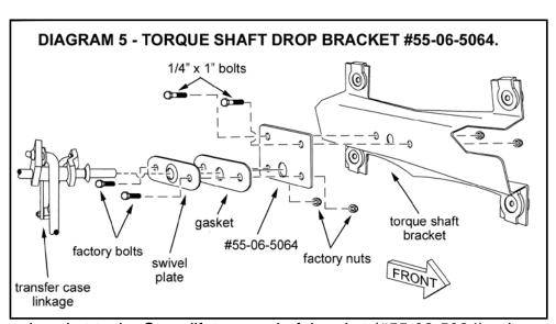
Attach the swivel plate and gasket to the Superlift torque shaft bracket (#55-06-5064) using the supplied factory bolts and nuts (18).
