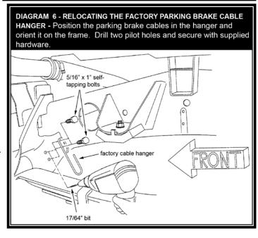
driver side parking brake cable in the lower hole in the "03" bracket. Be sure the prongs of the factory cable retaining clips are spread enough to secure each cable.
