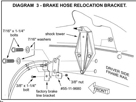
□□ Carefully bend the hard line down from the factory position and attach the factory bracket to the "10" and "11" bracket as shown using the supplied 3/8" x 1-1/4" bolt and nyloc nut (33).
