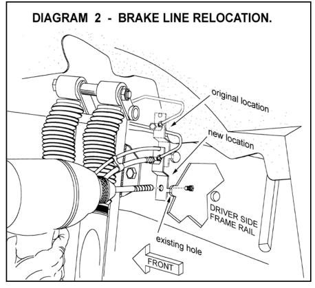
factory hardware and tighten to factory specs.
