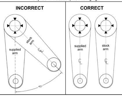
This can be accomplished by stacking the stock arm on the supplied arm (see DIAGRAM 1). The splines and indexing lugs must line up exactly. If a difference is noted (i.e. the pitman arms do not line up), contact Superlift before proceeding.
