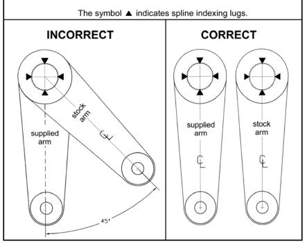
This can be accomplished by stacking the stock arm on the supplied arm (see DIAGRAM 1). The splines and indexing lugs must line up exactly. If a difference is noted (i.e. the pitman arms do not line up), contact Superlift before proceeding.
