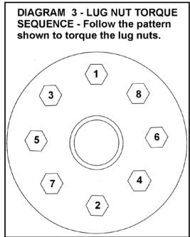
Install the lug nuts loosely. Tighten the lug nuts only until snug using the lug nut tightening pattern shown in [DIAGRAM 3] to minimize runout. The lug nuts are fully tightened in a later step.
