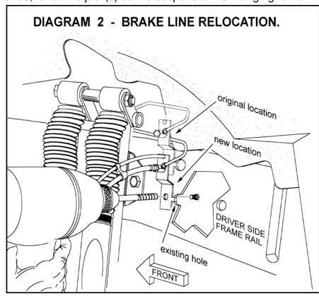
factory hardware and tighten to factory specs.
