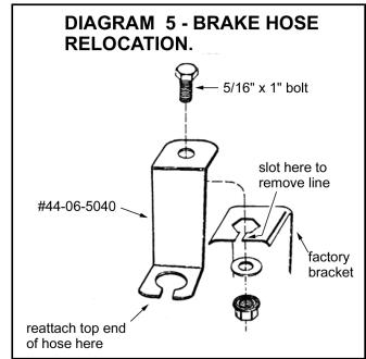
**NOTE:** The hard line will kink and collapse easily. Also, when routing, be sure the metal line does not make contact with the frame or any other components, or the line could eventually chafe through and fail.
