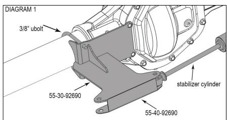
Install the supplied 3/8" x 3-13/16 x 5-1/2" u-bolt around the differential housing and through the "30" bracket as shown. Secure using the supplied 3/8" washers and nyloc nuts.
