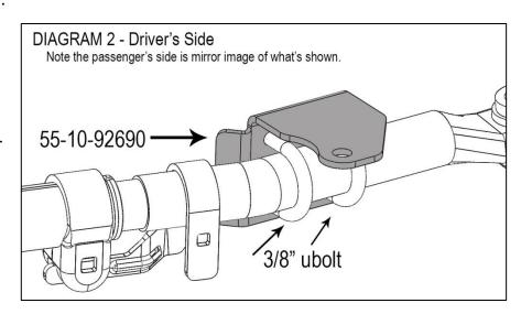
mounting hole on the "10" bracket. Make sure the top of the "10" bracket is level with the ground, then tighten the 3/8" nuts (26).
