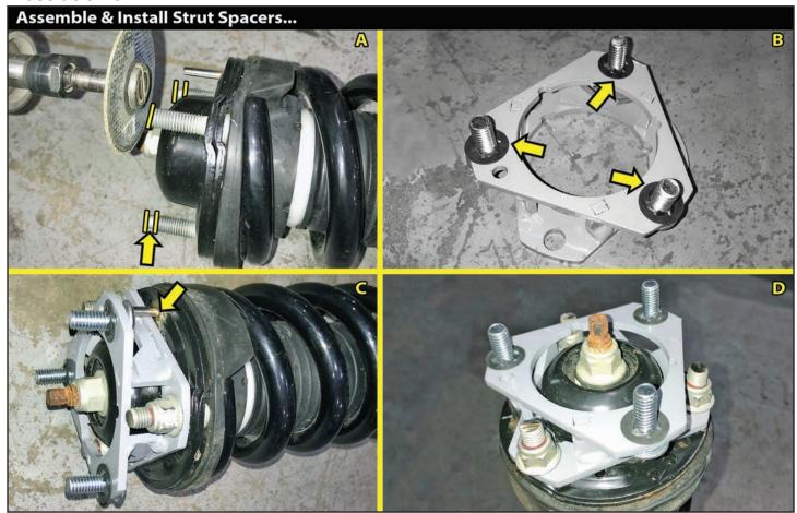
NOTE: Perform Steps 8-10 One Side At A Time. Start on the Driver Side & Complete Steps 8-10.
