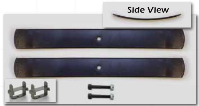
Universal Add-A-Leaf Kit Fits most vehicles with 2 1/4" Leaf Spring Assemblies Part No. 11-1070
