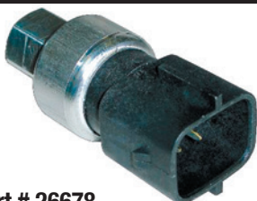
Part # 26678 Binary Pressure Switch Activation Pressure: 450 Deactivation Pressure: 265 Automotive Electrical Terminal Type: Spade FORD 2000-2008 MERCURY 1999-2008
