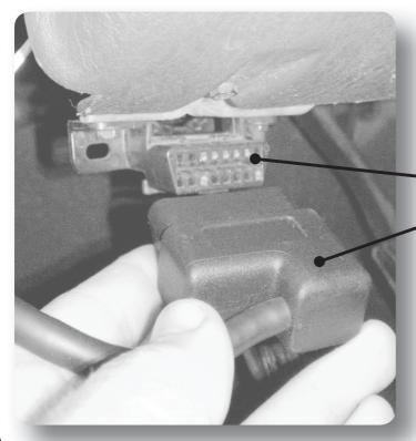
Next, locate the OBDII port underneath the dash. Plug the OBDII cable into the OBDII port.
