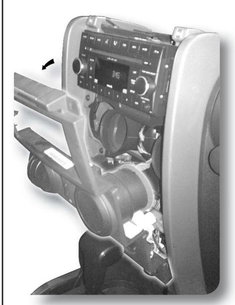
Starting from the top, pull the front panel back and away from the dash.
