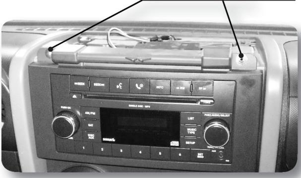
Remove these screws using a 7mm socket or wrench. Set aside.
