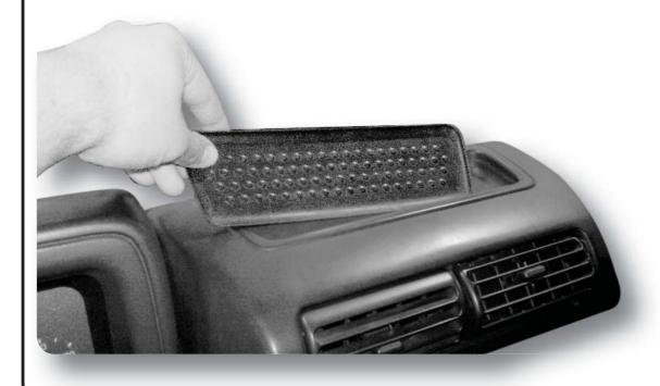
Remove the rubber insert located in the bottom of the dashtop tray. This will need to be removed in order for the pod to be properly fastened into place.
