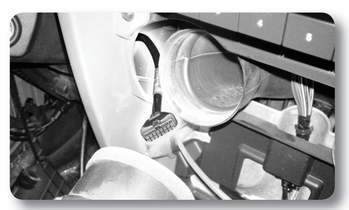
Route the cable from underneath the steering column, and through the side of the center panel area as shown.
