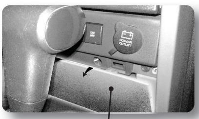
Remove lower panel using the screw driver method as shown in step 1 to expose the screws.
