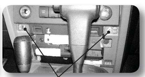
Remove the (2) screws shown using a 7mm socket or wrench.
