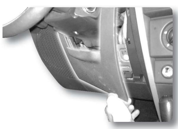
Next, remove the panel directly under the steering column.
