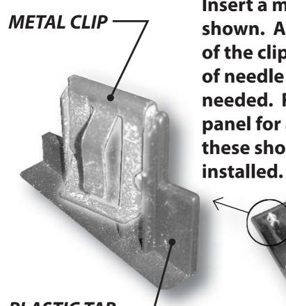
Insert a metal clip over each of the pod tabs as shown. Allow the small "teeth" on both sides of the clip to pierce into the plastic. Use a pair of needle nose pliers to help seat them if needed. Refer to the original
