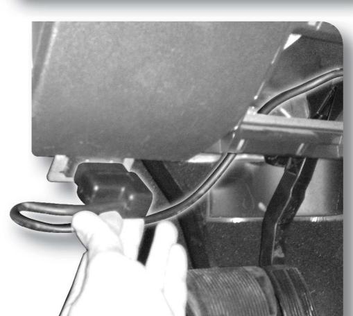
Next, route the cable up and along the side of the radio as shown.
