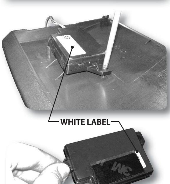
Using a Phillips head screwdriver, remove the compass module located on the bottom side of the panel you have just removed.
