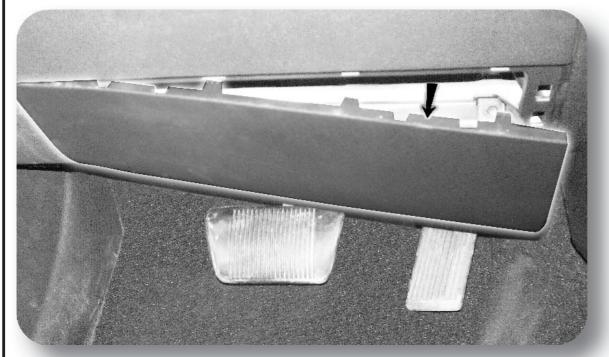
Remove the lower dash panel located directly above the foot pedals.
