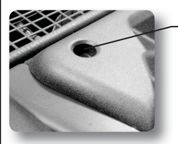
Next, using the provided self-tapping screws, fasten the pod to the dash. DO NOT OVERTIGHTEN
