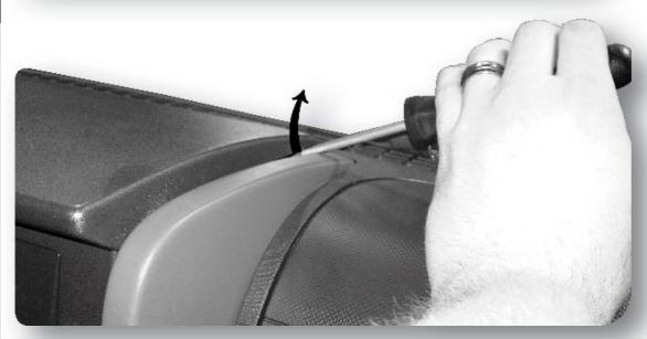
The panel is held in place by clips located on each side closest to the windshield. Insert a flat head screw driver underneath each side and pry up on the panel until the clip is released.
