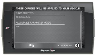
**NOTICE** *Do not remove or bump the OBD-II connector during any programming sequence. If you do, the vehicle may not start.*
