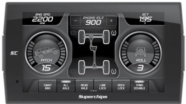
(1) PID's are displayed in the upper outer corners and can be setup to display any parameter you'd prefer by double tapping the PID itself.
