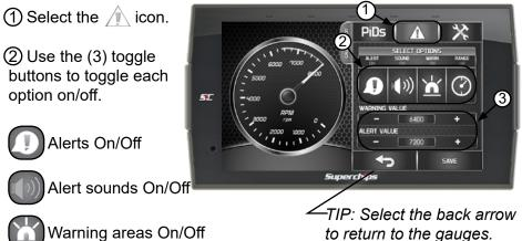
③ To adjust the warning and alert values for the PID, use the value editors. Tap on the center value to open a keypad to set specific values.
