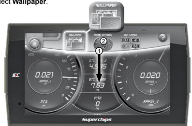
③ Toggle through the available background images by either swiping up/ down on the image, or using the up/down arrows.
