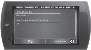
**NOTICE** Do not remove or bump the OBD-II connector during any programming sequence. If you do, the vehicle may not start.
