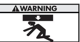
THIS IS A LIFTING DEVICE ONLY. DO NOT MOVE OR DOLLY THE VEHICLE WHILE ON THE JACK. IMMEDIATELY AFTER LIFTING SUPPORT THE VEHICLE WITH APPROPRIATE MEANS.
