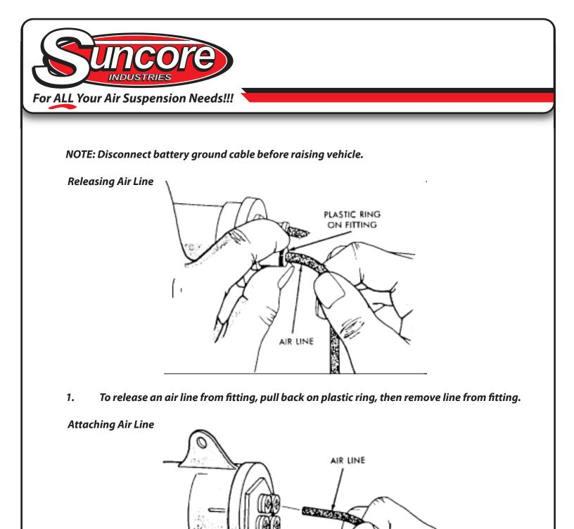
2. Air line fittings have a push-in feature. A brass type Colette locks the air line in place. One rubber O-ring seals the air line to prevent leakage. To attach air line, push into fitting.
