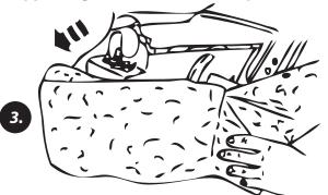
3. Inside the luggage compartment, position insulation out of the way from the shock absorber upper mount.
