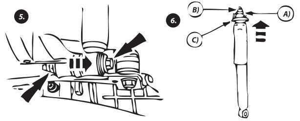
6. Separate the rear shock absorber insulator from the rear shock absorber.
