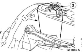
2. Seat the bottom of the air spring
