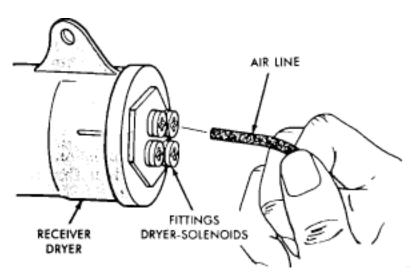
2. Air line fittings have a push-in feature. A brass type Colette locks the air line in place.
