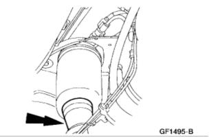
5. Lift the bottom of the air spring off the rear axle
