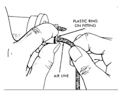
1. To release an air line from fitting, pull back on plastic ring, then remove line from fitting.
