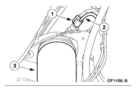
Connect the air spring solenoid valve.
