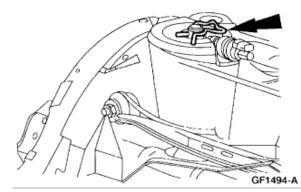
4. Remove the rear air spring retainer.
