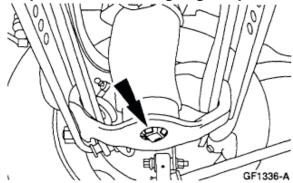
4. Lift the bottom of the air spring upward while depressing the locking tabs on the bottom of the air spring seat.
