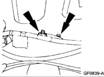
9. Remove the attaching nuts on top of the rear crossmember and remove the shock absorber.
