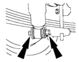
8. Remove the shock absorber lower retaining nut and bolt and swing the shock absorber out of the lower mounting bracket.
