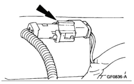
6. Remove the rear shock absorber electrical connector from the rear crossmember and disconnect the electrical connector.
