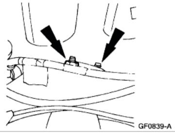
9. Remove the attaching nuts on top of the rear crossmember and remove the shock absorber.
