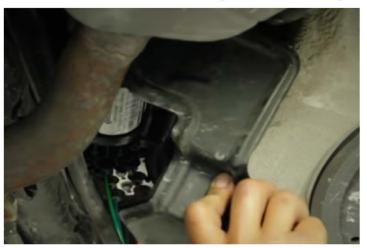
5. Disconnect 3 Electrical Plugs Along With Intake Hose From Compressor.
