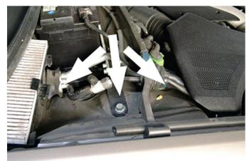
**2.** Remove the pinch bolt from the front of the control arms.
