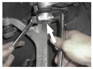
**3. Remove both ball joints from the front suspension link.**
