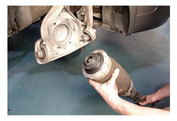
**9. Replace the cast aluminum shock cap and install the six (6) top mounting bolts.**
