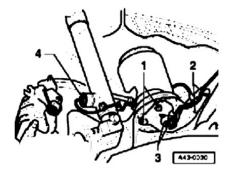
2. Carefully open and remove air connections (#4).
