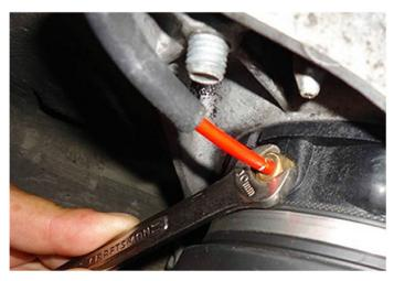
5. Loosen and remove the lower shock bolt.
