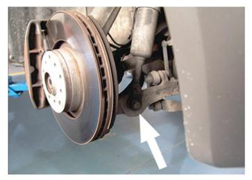
6. Carefully remove the air strut assembly from the vehicle.
