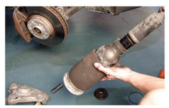
11. Remove and discard the old O-ring used to seal the air spring to the shock. This o-ring will not be reused in the new assembly.
