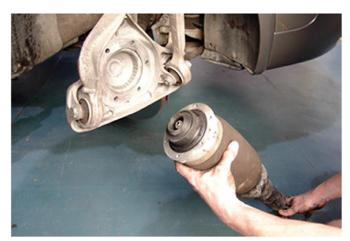
9. Remove the rubber upper mount and washer.
