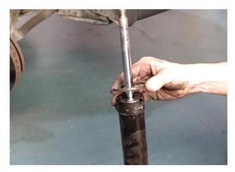
12. Lubricate the O-ring in the bottom of the new air spring assembly, and slide the new air spring over the shock absorber.
