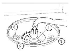
7. Remove locking clip (#1) from the bottom of the air spring and remove air spring assembly.
