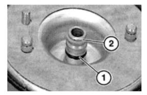
Check correct seating of sealing rings (1 - 2). **Note:**Do not under any circumstances grease sealing rings.
