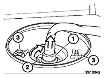
Press quick coupling (1) downwards, keep snap ring (2) pressed and detach quick coupling upwards. Attach protective cap to connection. Remove clips (3).
