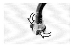
Plug-in coupling with snap ring.
