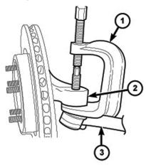
9. Remove the upper ball joint nuts and separate the upper ball joint (#2) from the knuckle (#3) using ball joint press.
