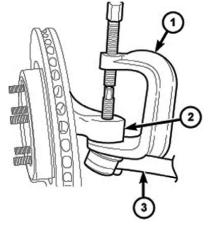
9. Remove the upper ball joint nuts and separate the upper ball joint (#2) from the knuckle (#3) using ball joint press.
