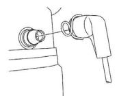
11. Remove the Lower Shock Mounting Bolt. Remove Shock From Vehicle.
