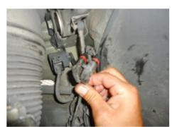
4. Cut the cable tie and remove the wiring bracket from the air strut.
