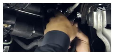
9. Remove Brass Fitting From Air Line by First Opening the Collett and Then Sliding Off. Push the Air Line in to the New Fitting Until it Bottoms Out.
