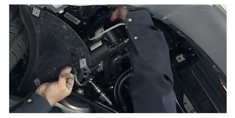
11. Verify the Air Line is Secure by Pulling Outward to Feel Resistance.
