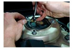
6. Remove the three nuts on the upper strut mount to the frame.
