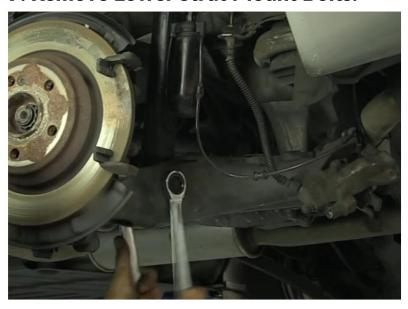
10. Pull Downward on the Lower Control Arm to Free Strut Assembly. Remove Strut From Vehicle.
