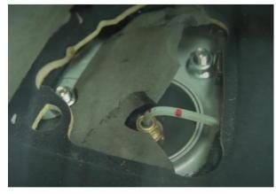
3. Remove Air Fitting From Top of Strut.
