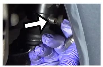
6. Separate Upper Control Arm Ball Joint from the Spindle Assembly. Remove Strut Assembly.
