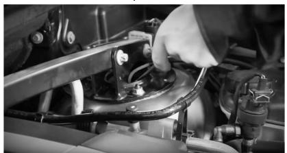
3. Remove Brass Fitting From Air Line By FIrst Opening the Collett and Sliding Off
