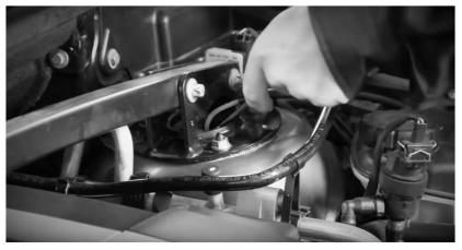
3. Remove Brass Fitting From Air Line By FIrst Opening the Collett and Sliding Off
