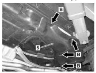
2. Remove cover (#5) and unscrew four plastic nuts (Arrows B).
