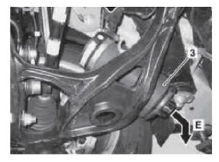
6. Remove air spring (#3) downwards at an angle (Arrow E).
