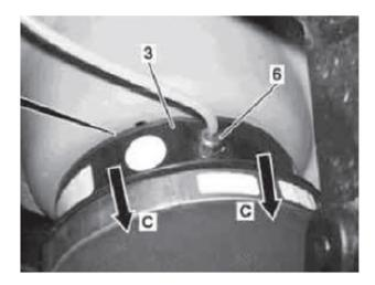
3. Unscrew threaded connections of air suspension pressure line (#6) from the air spring (#3).
