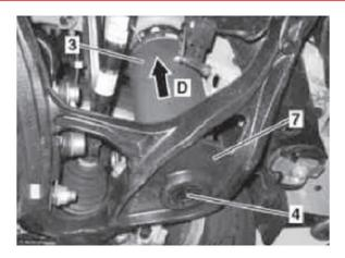
5. Carefully push the air spring (#3) together (Arrow D), in the process press the air spring centering (#4) out of the spring control arm (#7) from below.
