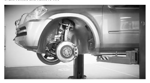
6. Remove Retaining Nut and Disconnect Wire to Strut if ADS is Installed
