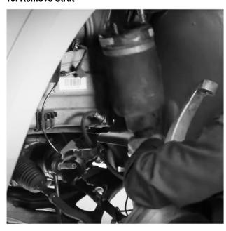
11. Remove Air Fitting. Tap on Center Cap to Gain Access to the Metal C-Clip. Use a Flat Head Screwdriver to Remove C-Clip From Top
