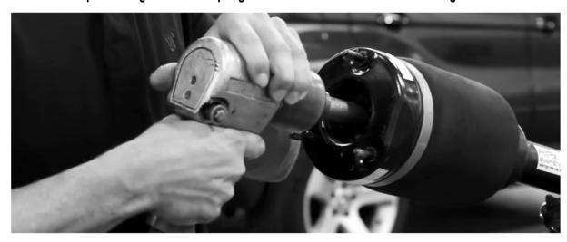
14. Install Flat Rubber Ring and Then Round O-Ring Down the Shock. Lubricate New Rubber. Slide New Air Spring Over the Shock
