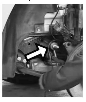
9. Use Jack to Take Pressure Off of Lower Arm. Remove Lower Strut Mount Bolt
