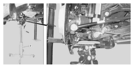
7. Raise the suspension with telescoping transmission jack (#2) and passenger car transmission platform under the supporting joint (Arrow A) far enough until the suspension is slightly deflected.
