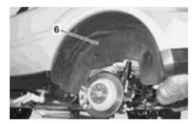
5. Remove fender liner in rear fender (#6).
